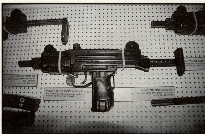
A 9mm Mini-Uzi variant from 1982 not adopted for service. Note two-bar telescopic stock but this time no pistol grip.
