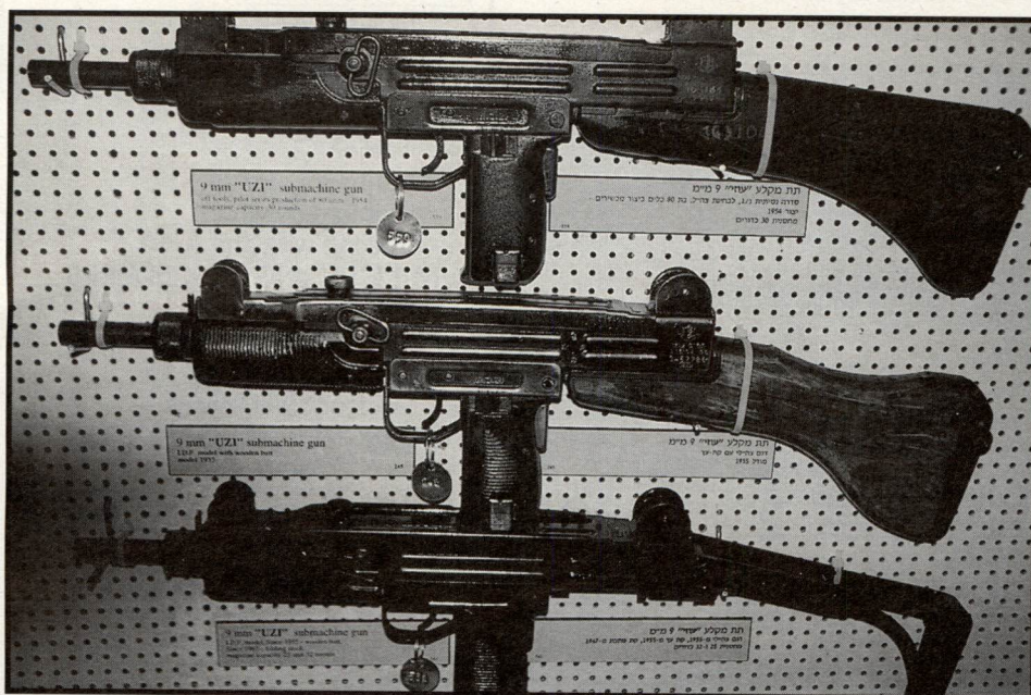
A close-up from top to bottom. A: One of the 80 pilot series 9mm Uzis issued to army units for testing and suggested improvements in 1954. Magazine 30 rounds. B: Standardized 9mm Uzi issued for service in 1955. Magazine capacity now 25 or 32 rounds. C: 1967 Model 9mm Uzi now equipped with a folding metal stock.
