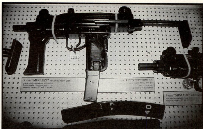
9mm Mini Uzi, 1982, in a prototype form not adopted for service. Note front pistol grip and the one bar telescopic stock. Fitted with a 32-round magazine.
