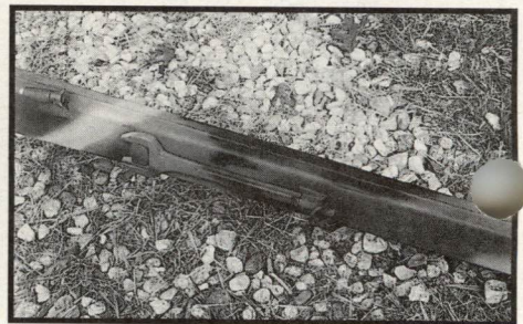
Picture 5: The right trail leg carries the muzzle brake wrench and cleaning rod.
