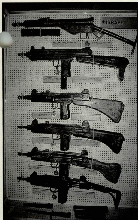
A line up of Israeli made submachine guns. From top to bottom: A: A 9mm Sten clone circa 1944, 32-round magazine built of inferior materials by the Hagana, the underground Israeli Army before statehood. B: The first ever Uzi 9mm prototype built as a tool-room model in 1951. Magazine capacity 30 rounds. C: One of the five early 9mm Uzis submitted for the competitive trials in 1952. Magazine 30 rounds. D: One of the eighty pilot series 9mm Uzis issued to army units for their suggested improvements in 1954. Magazine capacity 30 rounds. E: Standardized 9mm Uzi issued for service in 1955. Magazine capacity now 25 or 32 rounds. F: 1967 model 9mm Uzi now equipped with a folding metal stock.
