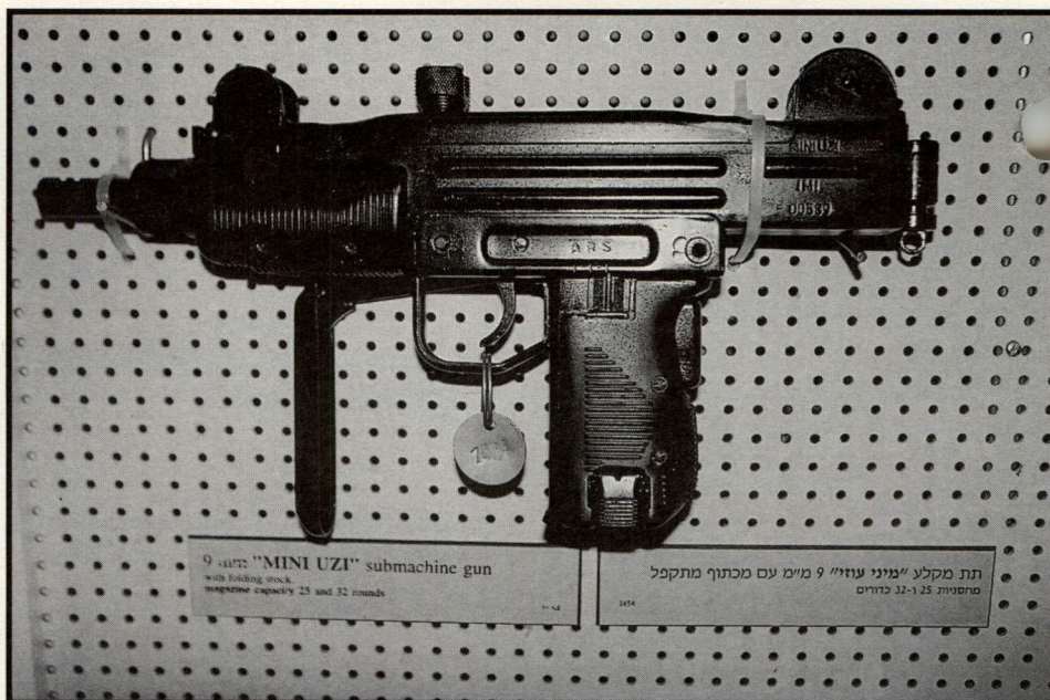
9mm Mini-Uzi with folding stock as accepted for service in 1982. Stock folded. Magazine capacity 25 and 32 rounds.
