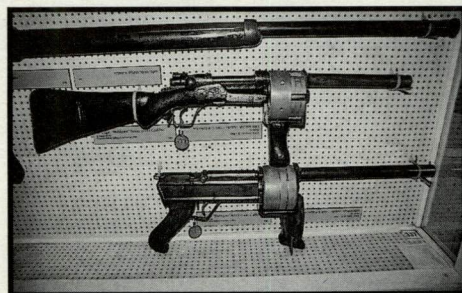
The dubious, Dubigun a 12-gauge "carbine" built as an act of desperation in a secret workshop on Kibbutz Ein Gev in 1946. The weapon has a six-round drum magazine.
