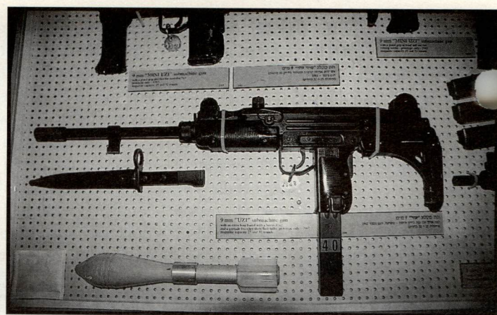
Uzi with attitude! An Uzi fitted with an extra long barrel, bayonet lug and grenade launcher. Note flash hider at end of the muzzle, the bayonet, and the formidable looking grenade below the gun. A one-off prototype 1967.
