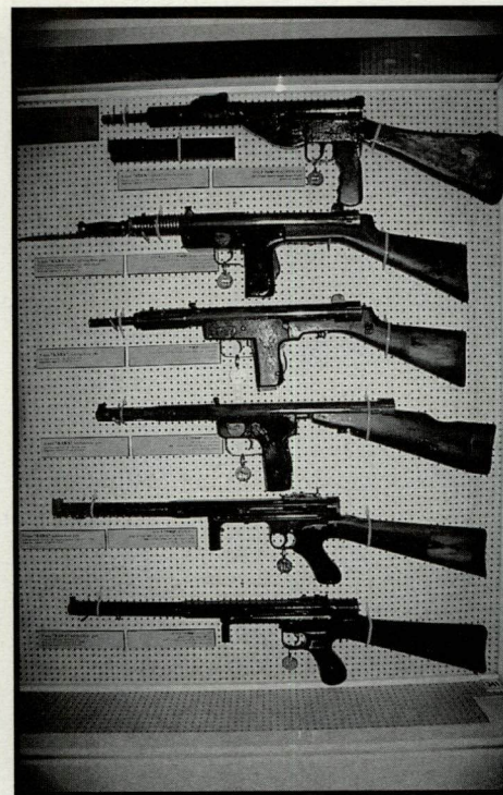
From top to bottom. A: A 9mm Sten clone, this time built by a secret factory owned by the Stern Gang terrorists. B: 9mm Kara Model K-12, the final prototype Kara which was submitted in competitive trial against the first Uzi. IDF Service Corps development 1951. Magazine capacity 20 or 40 rounds. Note the gun is fitted with a bayonet! C: 9mm Kara prefinal prototype developed in 1950. Magazine capacity 20 or 40 rounds. D: 9mm Kara prototype 1949 version. E: 9mm Kara early prototype 1948 version. Note at this early stage, the Kara did not have its magazine housing in the pistol grip. F: 9mm Kara early prototype from the same period with minor modifications.
